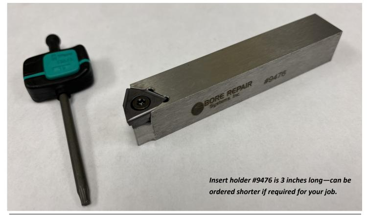
The Bore Repair Systems, Inc. Ultra-Carbide indexable line bore cutter kit is our newest design in cutting bit kits.
