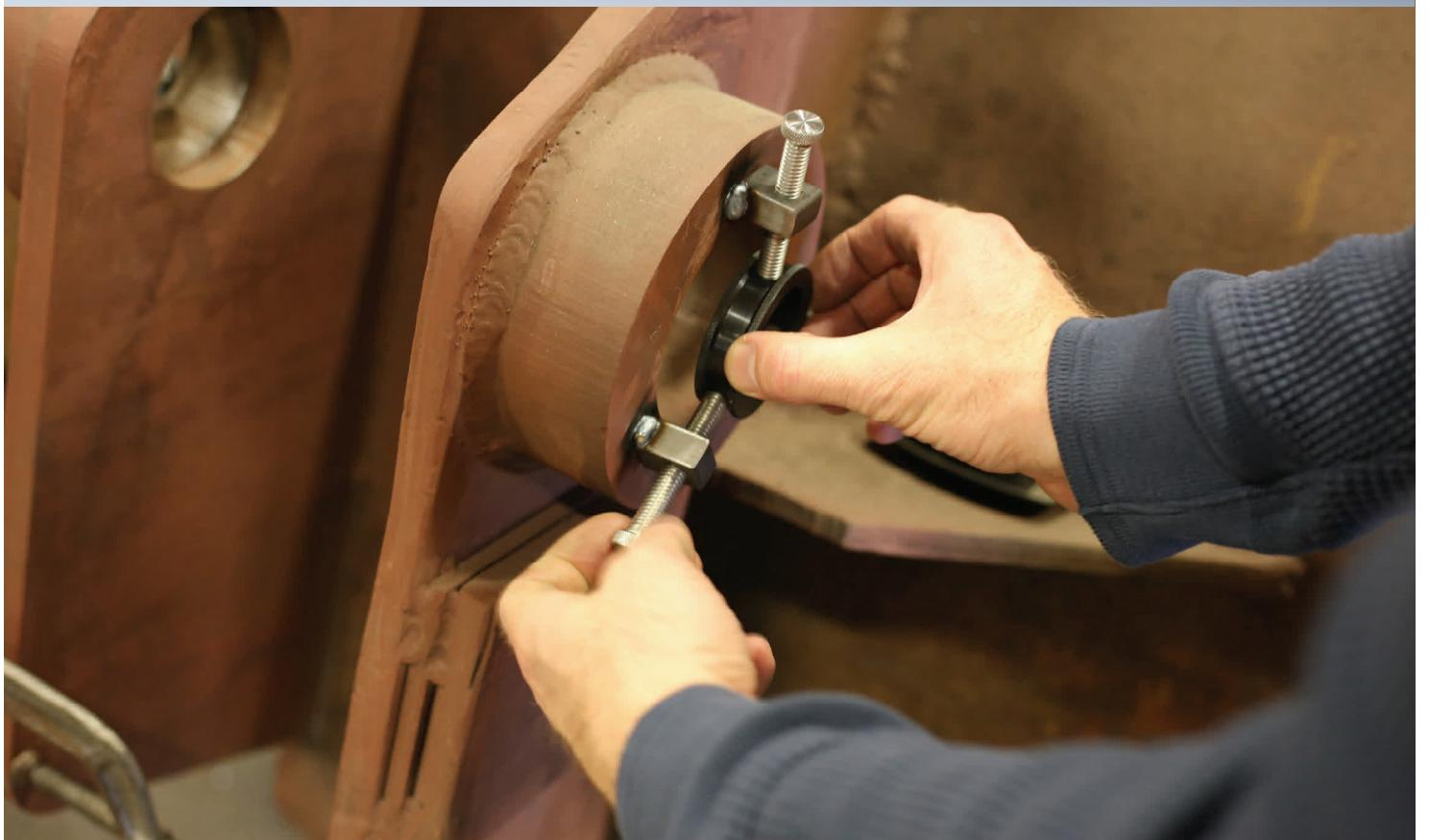
**Rotate ring so the tapped holes are between screws**
