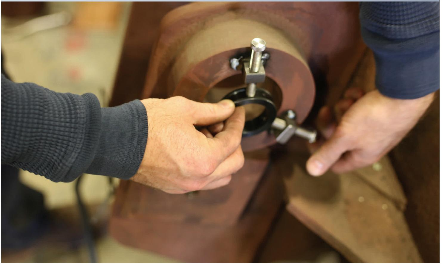
**Re-tighten the centering screws to retain the ring**
