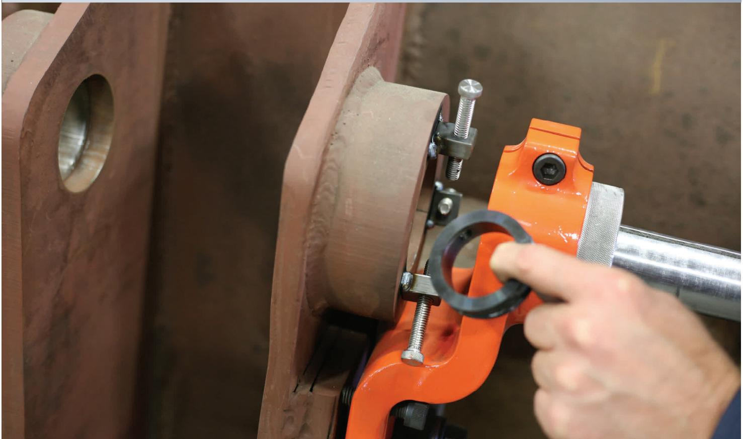
**Leave centering tabs and screws if desired. This will allow easy re-centering if you find that bar still needs further adjustment.**
