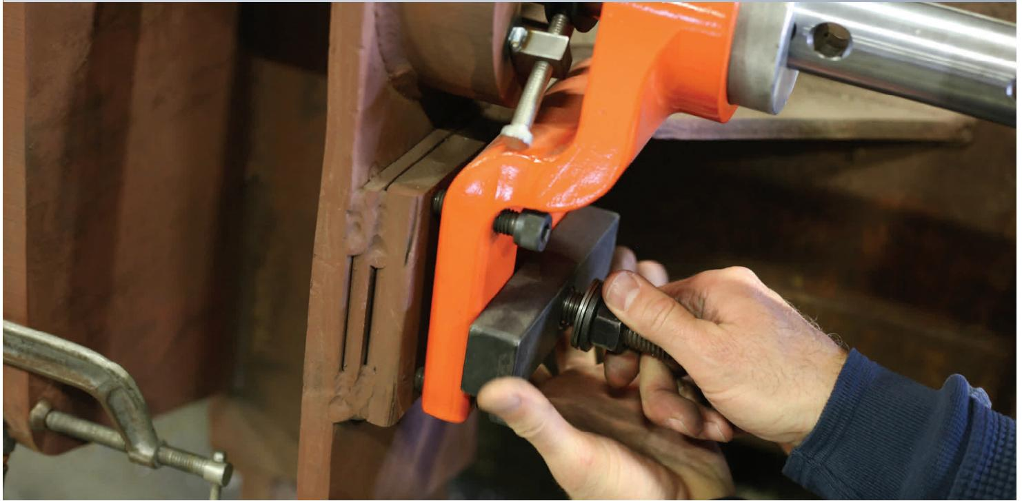
**With both mounts attached to job, loosen screws**
